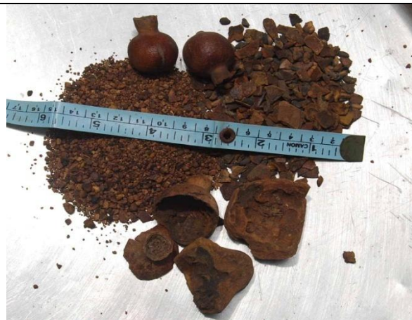
Fig-4a – Size reduction of the punica rind, bone dried-stone hard; excellent keeping quality at room temp (tropical humid).
